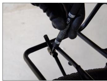
Mark the stays ca 10mm over where they exit the eyebolt drilling. Take the stays off the rack and cut them where you marked them. File or sand the stay ends and remove all burs or sharp edges.
