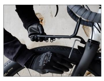
Select the right length M6 bolt which fits best your specific fork crown. Insert bolt into the rack attachment barrel, fit the spacers and then screw the rack loosely to the fork crown. Do not tighten it up now.
