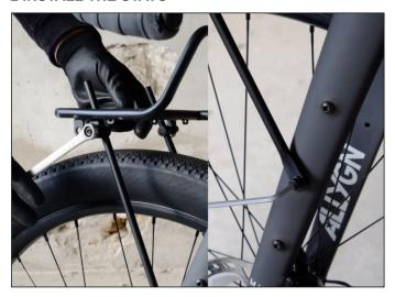
Install the rack stays to the rack as shown on the illustration on the left page. Then mount the stays to the midfork eyelets. Fasten the screws loosely at this point, so you can still adjust the racks angle at this point.
