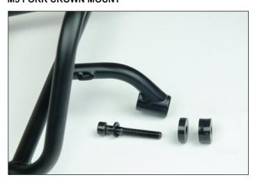
If your fork has an M5 fork crown mount then use the M5 bolt and washer. If needed, use one or more plastic spacers and select the right length of bolt. Please use Loctite 243 medium tight or similar!
