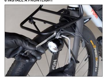
If you have a frontlight which can be mounted upside down then just mount it to the light tab on rack using the M5 22mm bolt, washers and nuts.
