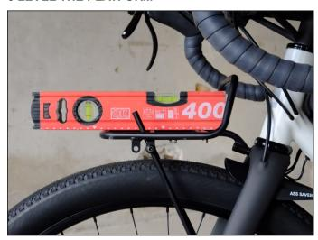
Check in side view if the rack is level to the ground. Use an spirit level if you have one. Adjust the rack angle in front view and check if it's level relative to the headtube. Check side view again and re-adjust if necessary.
