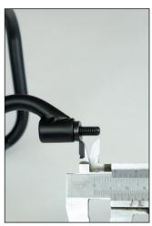
On carbon forks the fork crown mounts are usually deadend threads so it is very important not to use bolts that are too long as this can result in damaging the mounting point and/or the fork itself. Measure how far the thread goes inside and select the length of bolt accordingly!
