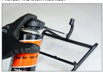
If you live in very moist and wet areas, especially close to the sea, we highly recommend to use some spray lubricant like WD40, Fluidfilm, Mike Sander, etc inside the rack. Simply spray a good amount inside every venthole at the backside of the rack before installation. Move the rack around and let excess oil come out of the ventholes. Keep in mind oil might be dripping from the rack even after some time, so don't park the bike on your most fancy carpet at home;)
