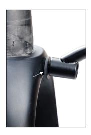
Especially on carbon forks it is important to protect the fibres from damage. On other material forks the rubber washers may help to protect the paint and make it easier to adjust the rack angle. Please always use protective tape between the rubber washer and the fork mounting points to make extra sure the paint will not be damaged. Please use Loctite 243 medium tight or similar!
